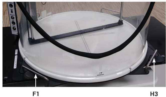
Fig. 2: 3D SCANNER placement within CPP
