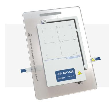
Calibration fixture included with every Daily QA-MR for device calibration.
