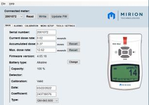
CSW-Med software for advanced configurations of the RDS-Med Survey Meter
