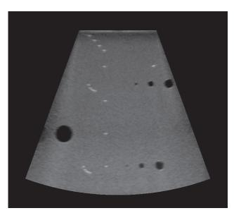
Our proven Sono403 Phantoms have precision-placed targets.
