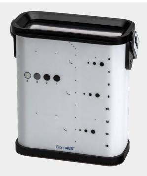
Sono403 Phantoms, with patented HE (High Equivalency) Gel™, provide advanced technology for measuring image quality of small parts and intra-cavity ultrasound scanning systems.
