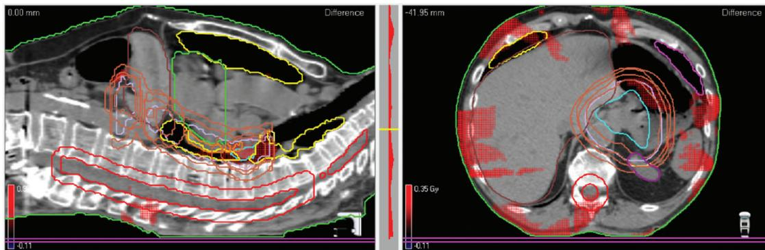
Figure 3. Difference colorwash, based on DoseCHECK calculation, indicates regions above 3% of the maximum dose for a commissioned TPS (errors with off-axis softening). There are only overdosed regions, some of which fall in organs at risk such as the spinal cord. The target region (light blue contour) indicates no differences beyond 3%.
