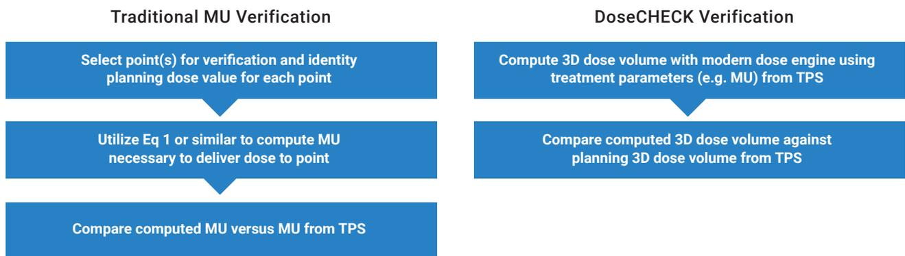
Figure 2. Comparison of secondary calculation workflows for: a) traditional MU calculations, and b) full 3D volume verification (e.g. DoseCHECK)
