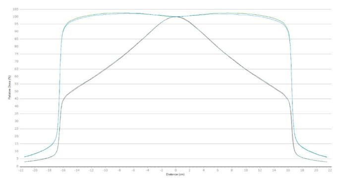
Crossline profiles for 30 x 30 cm<sup>2</sup> field in 10 MV and 10 MV flattening-filter-free beams for both systems. There is a difference of less than 1% in dose between the machines.
