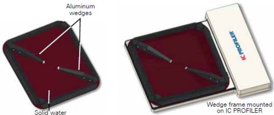
Figure 2: Aluminum double wedge for electron measurements
